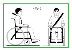
Pelvic restraints should make full contact across the front of the body near the junction of the thigh and pelvis
