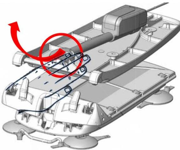
Lift from this part only to remove the backrest from the base of the Aqua Bath Lift.
